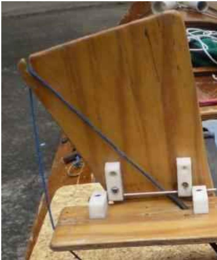
*Fig 6. This shows where the rudder line goes to, from where it exits the black tubing, round the hinge pin, up the front of the pedal and through the hole (slot) at the top. From there it goes aft to the rudder – bit of line shown dangling in this picture.*
