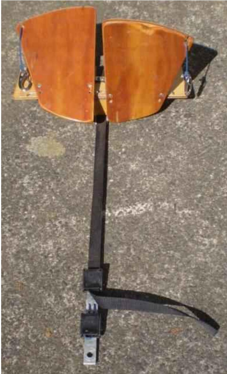
*Fig. 9 Complete unit from the paddlers view. Note second camlock for the rudder-lines which run under the bar to the front end of the bar then back through the platform tubes, round the hinge pin and out of the hole at the top of the pedals. The lines from the pedals are attached to the lines to the rudder by clips.*
