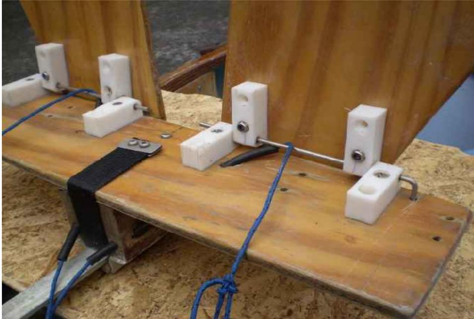
*Fig 5. Assembled looking at the front of the pedal unit. This shows the hinges and retaining strap. Ignore the second holes in the hinge blocks, only one 4 mm bolt is necessary.*
