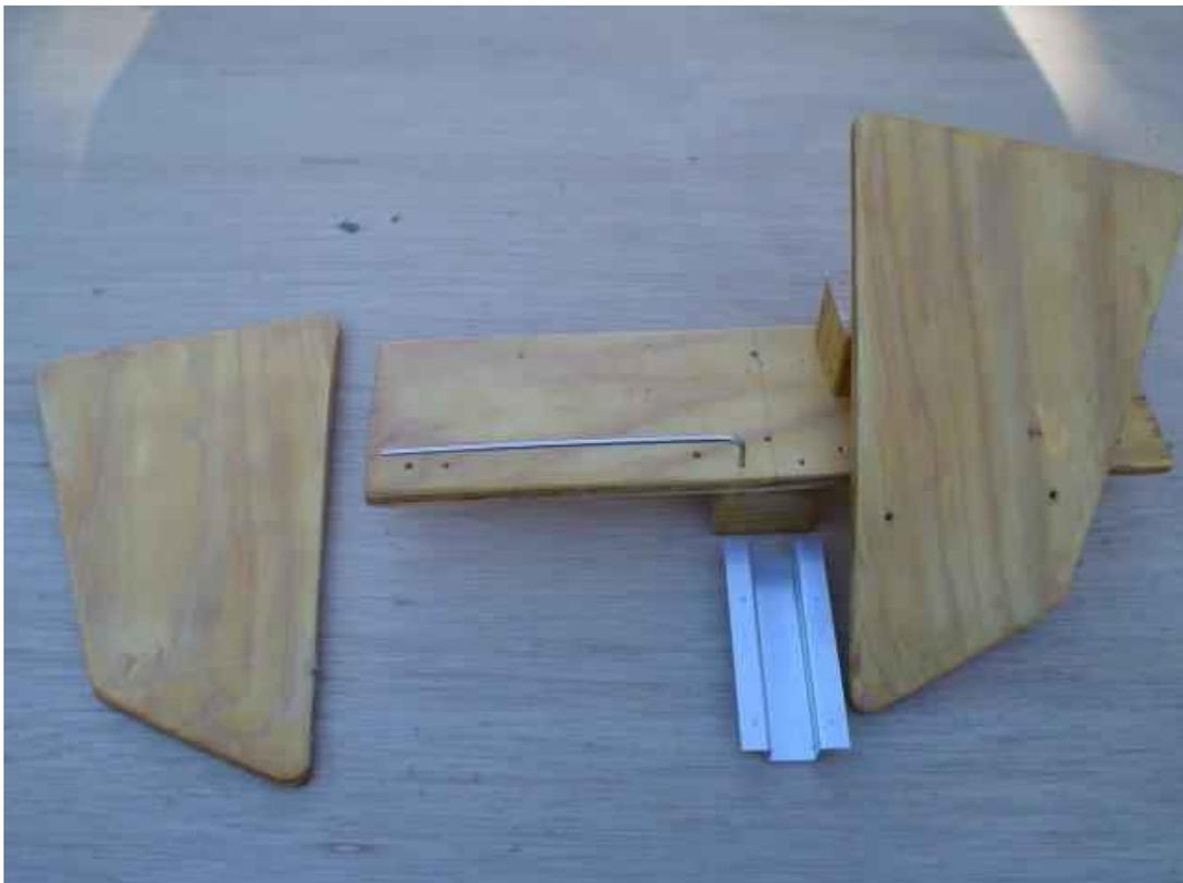
*Fig 3. Left to right, pedal, platform with hinge pin, top-hat section to hold the platform on the bar under the platform and right pedal roughly in the position it will be mounted. Note the hinge pin is bent and fits into a hole in the platform. This is to stop it sliding out of the hinge blocks..*
