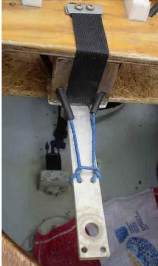
*Fig 7. The rudder line can be fastened to the bar or taken back to another camlock to allow pedal angle adjustment. This unit had a front bolt to hold the bar.*
